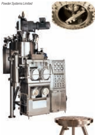
FIGURE 2. The Agitated Nutsche Filter Dryer allows the user to control and optimize the isolation by filtering out a maximum of the solvent using pressure and heated agitator blades to bring down the moisture content
