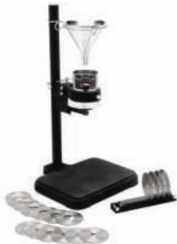
FIGURE 2. The flow cup test is relatively easy to setup and perform, and the data are used to calculate the Carr index, Equations (1), and Hausner ratio, Equation (2)
