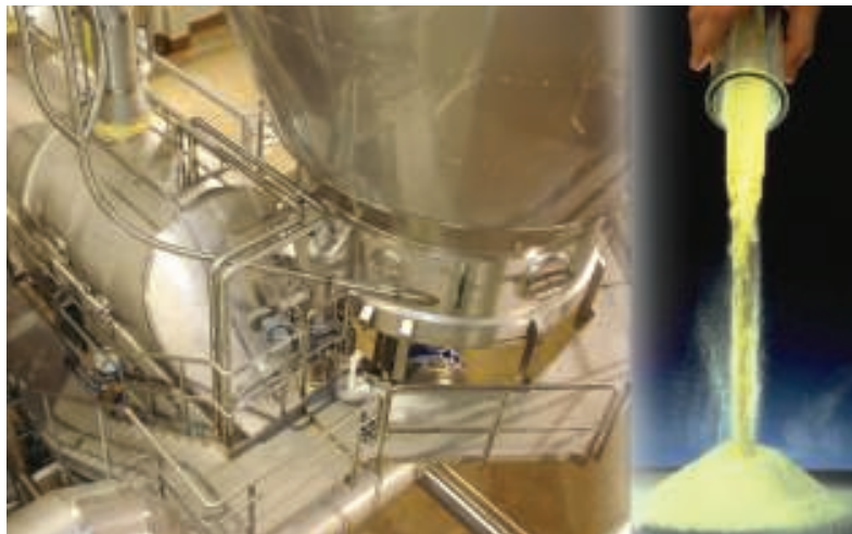
FIGURE 3. High- and low-viscosity liquids and heat-sensitive products should be spray dried because it is a continuous process, converting a pumpable liquid into a particulate matter in a single operation via spray dryers such as the Anhydro spray dryer shown here
