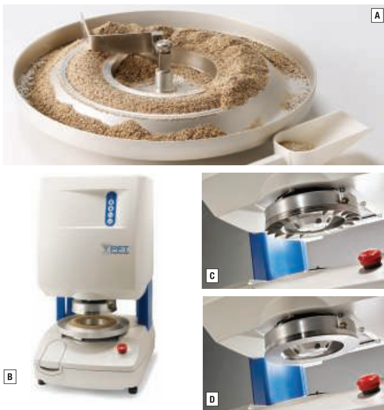
FIGURE 3. For shear-cell testing, powder is placed into a ring-shaped trough for annular shear cell (3a), which is placed into a commercial powder flow tester (3b), which uses either a vane lid (3c) or a wall-friction lid (3d)
