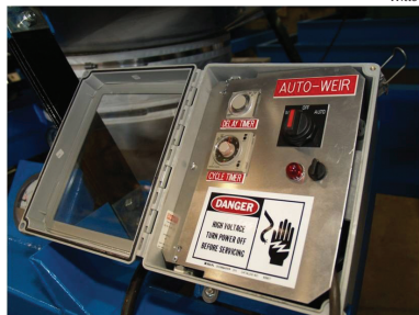
FIGURE 4. Witte's air-operated gates rotate 90 degrees above the deck on a cycle timer, allowing a pre-determined amount of product to advance, providing the operator with flexibility and realtime control over the flow and retention time
